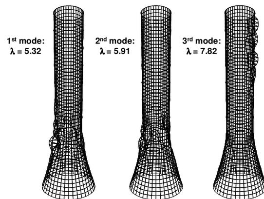
Figure 6: Buckling modes of 1000 m solar chimney
