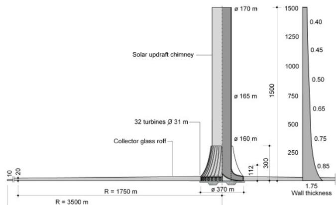
Figure 4: Overview over components of a SCPP
